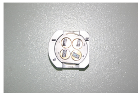
Figure 2: Wire Samples Being Loaded Onto the Studs
